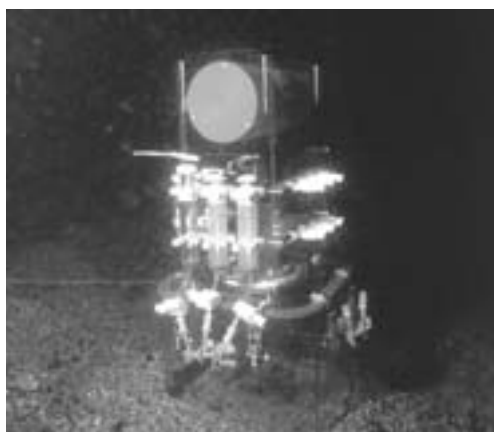
ABOVE FIGURE 1: Benthic flux chamber used for in situ measurements of oxygen and nutrient fluxes in sediments in Loch Creran
